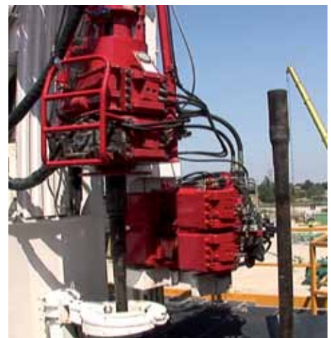
Torque wrench, hydraulic power tong and automatic slip
