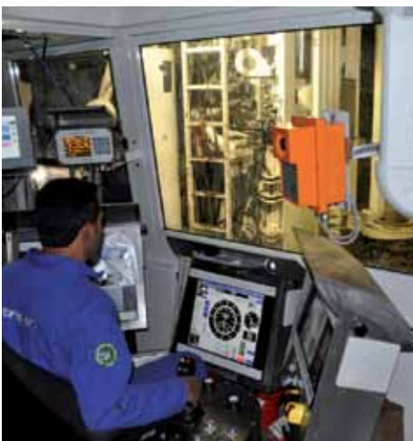
Cyber drilling console on a HH220 EC Rig
