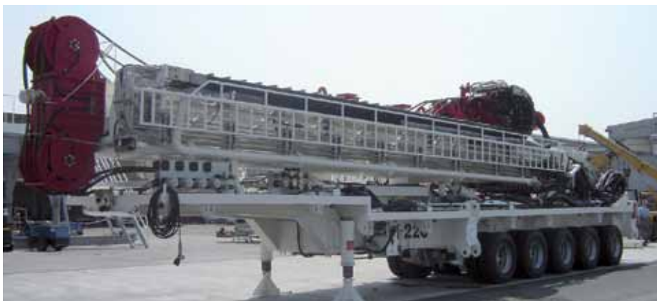
Mast on trailer for fast moving
